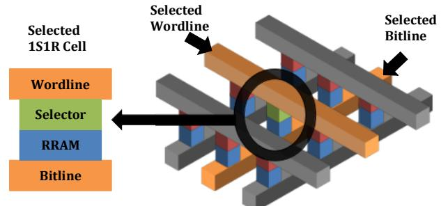
Fig. 2. Schematic of a 1S1R crossbar array.
