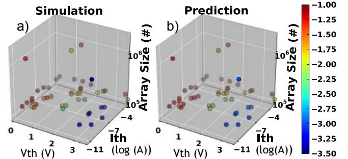
Fig. 6. Simulation (a) and prediction (b) results of IS1R array (512×512 and 1024×1024) RESET power consumption for test data. The color scale represents the logarithm of power consumption ( $\log(W)$ ). The unit of  $V_{th}$  and  $I_{th}$  is V and  $\log_{10}(A)$  respectively.
