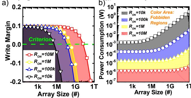
Fig. 8. (a) Envelope of write margin attainable by using optimal selector characteristics. For each RRAM with different LRS, the corresponding color space of write margin can be attainable by varying selector characteristics. (b) Envelope of energy consumption not attainable by using optimal selector characteristics. For each RRAM with different LRS, the corresponding color space of energy consumption cannot be attainable by varying selector characteristics.
