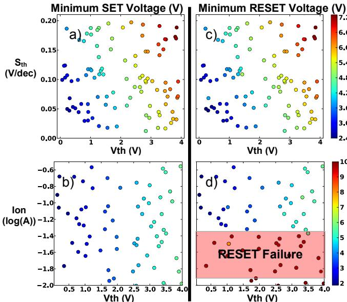
Fig. 5. Simulation results of minimum SET and RESET voltages for IS1R cells (absolute value shown by the color scale (V)): (a-b)  $V_{MINS}$  and (c-d)  $V_{MINR}$ . For (a)(c),  $I_{th} = 1 \text{ pA}$ ,  $I_{on} = 100 \text{ mA}$ , and  $S_{on} = \infty \text{ V/dec}$ ; For (b)(d)  $I_{th} = 1 \text{ pA}$ ,  $S_{th} = 0.01 \text{ V/dec}$ , and  $S_{on} = \infty \text{ V/dec}$ .
